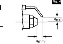
When re-installing the electrode holder, there must be a gap of 9mm between the electrodes and the nozzle (see fig. 4). If this adjustment needs to be re-set, it is preferable to remove the burner head complete, by removing the securing screws around its' edge, taking care not to damage the photocell. The electrodes may then be adjusted to their correct clearance before replacing the Burner Head.
