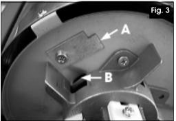
The blanking plate is factory set to burn PARAFFIN, so that tab'A' covers vent 'B'
