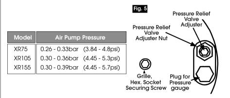
To adjust the pressure, insert an Allen key into the hex socket in the end of the Relief Valve Adjuster, and undo the Adjuster Nut. Turn the Allen key clockwise to increase pressure, and anticlockwise to decrease. Tighten the securing nut when the correct pressure is reached, ensuring the Allen key does not turn in the process.
